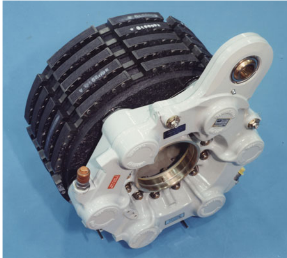
Fig. 8.8 A carbon/carbon brake assembly used on a Boeing 767 airplane [Courtesy of Allied-Signal Corp.]
