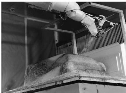
FIGURE 6.28 Robotic spray-up process for making a bathtub. The robot is applying chopped fiberglass with gel. (Courtesy of Fanuc Robotics.)
