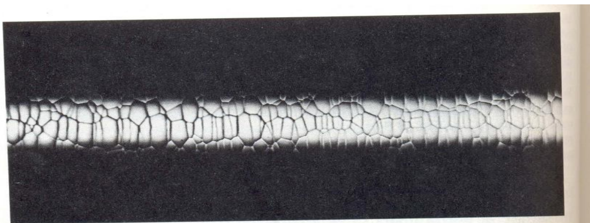
Fig. 3.9 Surface of boron fiber on tungsten substrate showing a corn-cob structure consisting of nodules (courtesy of Philips Co.).
