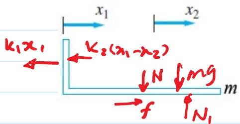
$$\sum F_{x_1} = m \ddot{x}_1 \Rightarrow -k_1 x_1 - k_2 (x_1 - x_2) + f = m \ddot{x}_1 \quad (3)$$
