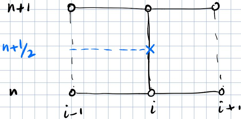
$$\frac{u_i^{n+1} - u_i^n}{\Delta t} = \frac{u_{i+1}^{n+1/2} - 2u_i^{n+1/2} + u_{i-1}^{n+1/2}}{\Delta x^2} + O(\Delta t^2, \Delta x^2)$$
