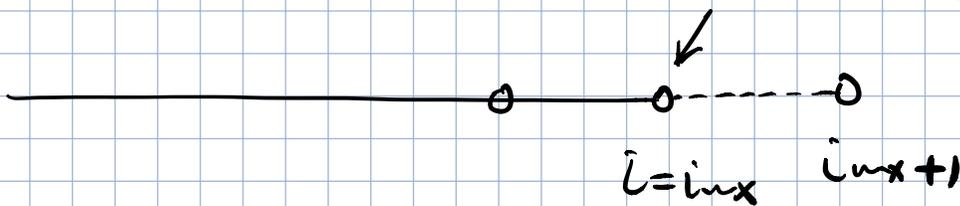
$$\left. \frac{\partial u}{\partial x} \right|_{i=i_{n+1}} = \frac{u_{i_{n+1}+1} - u_{i_{n+1}-1}}{2 \Delta x} = u_{nb}$$
