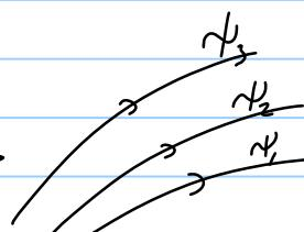
$$d\phi = 0 \Rightarrow \underbrace{\frac{\partial \phi}{\partial x}}_u dx + \underbrace{\frac{\partial \phi}{\partial y}}_v dy = 0$$
