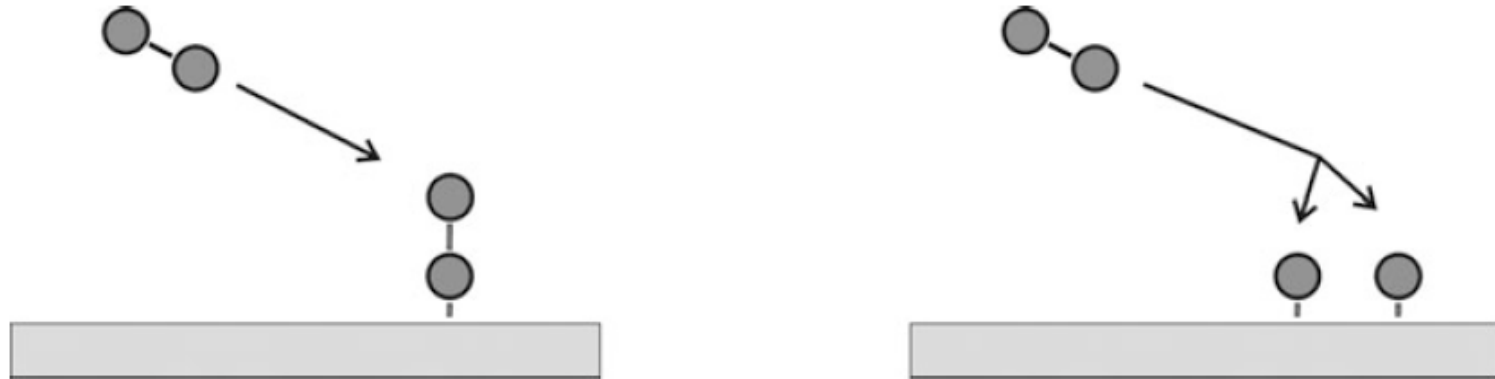
Fig. 3 Gas adsorption on a solid: physisorption ( left ) and chemisorption ( right )
