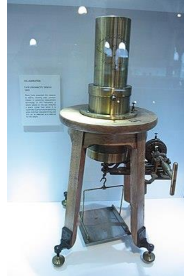
Piezoelectric balance presented by Pierre Curie to Lord Kelvin , Hunterian Museum, Glasgow
